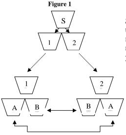
Sample (S) is an amount greater than or equal to twice the mass needed for testing. Sample (S) is reduced in a mechanical splitter to yield parts (1) and (2)
