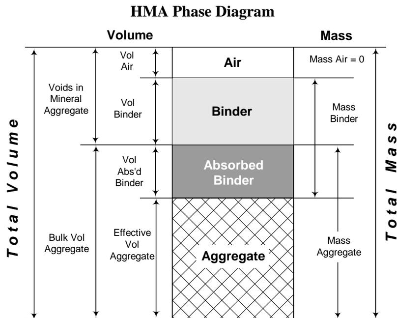
Each of the properties in the HMA phase diagram can be measured or calculated. For example: The mass of the aggregate is measured; the voids in mineral aggregate (VMA) is calculated; total asphalt binder can be measured but the amount available to act as a binder in the mix must be calculated because it is the quantity left after the aggregate has absorbed some of the asphalt binder.
