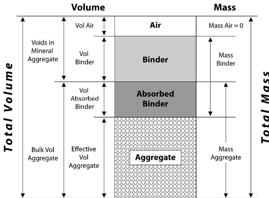
Each of the properties in the asphalt mixture phase diagram can be measured or calculated. For example: The mass of the aggregate is measured; the voids in mineral aggregate (VMA) is calculated; total asphalt binder can be measured but the amount available to act as aan effective binder in the mix must be calculated because it is the quantity left after the aggregate has absorbed some of the asphalt binder.
