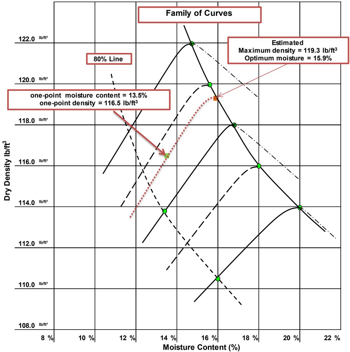
The results of a one-point determination were 116.5 lb/ft<sup>3</sup> at 13.5 percent moisture. The point was plotted on the reference curve graph. The point was plotted on the appropriate family between two previously developed curves near and intermediate curve.
